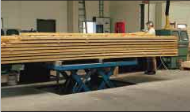
To reduce workforce back injuries this 4 tonnes capacity double horizontal scissor lift table is used to raise the load to an ergonomically correct height for onward handling.
