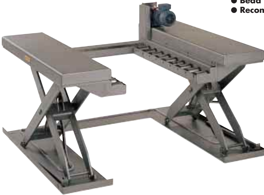
A specially built 1,200Kg capacity lift table with powered roller track. It is made for the food industry from EN 1.4301 stainless steel (normal stainless steel 18/8).
